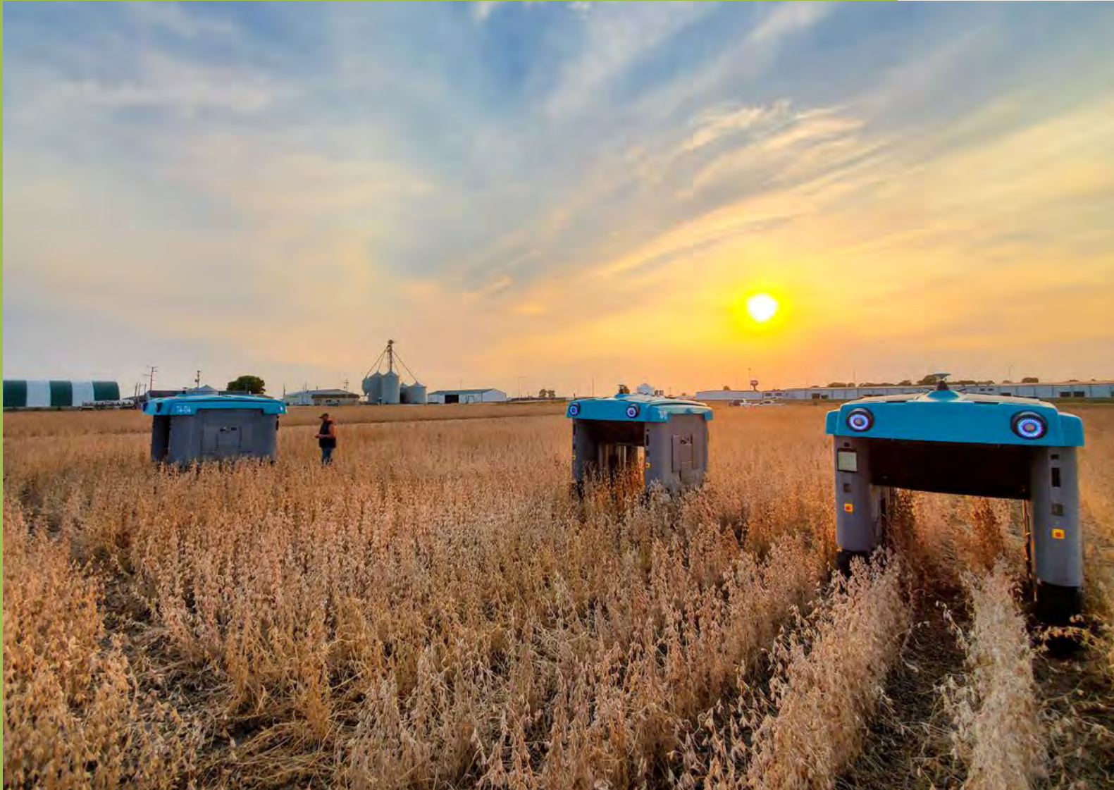
Mineral's plant buggy, a crop-inspecting robot, is being developed by Google's X, the Moonshot Factory research facility
